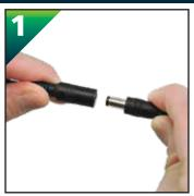
Insert adaptor jack into the plug on the left side of the unit.
