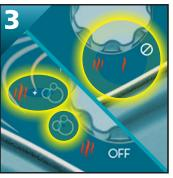
Turn the right knob to select your desired temperature setting. Turn the left knob to 1 or 3 for heating.
